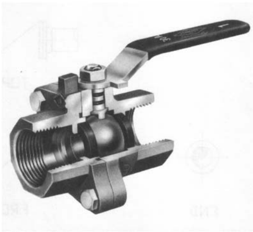
FIGURE 5.12 Ball valve. Courtesy of Jenkins Bros.
