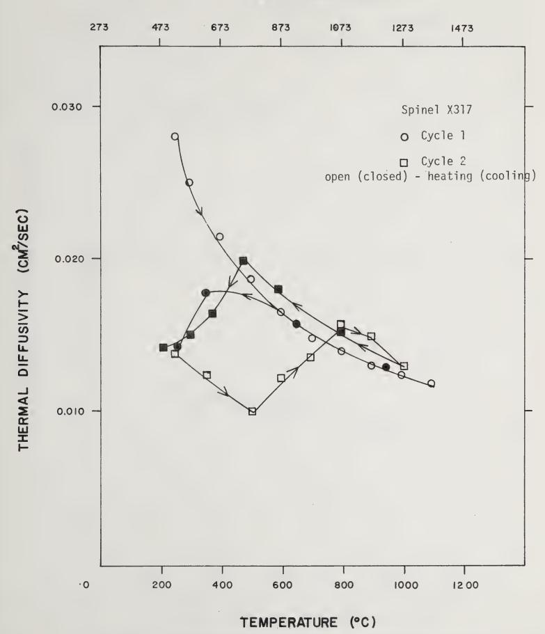
Figure 2. Effects of thermal cycling on the thermal diffusivity of as-fabricated fuel cast spinel refractory
