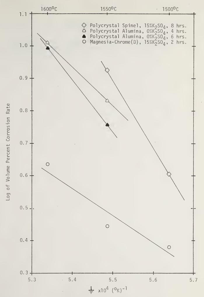
Figure 1. Plot of the logarithm of the volume percent corrosion rate versus the reciprocal of the absolute temperature for polycrystalline spinel and alumina, and for a commercial magnesia-Chrome, in air and at a dipping rate of 25 cpm.
