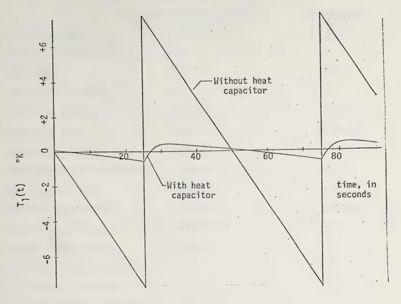
Figure 4. Variations in preheated air temperature
