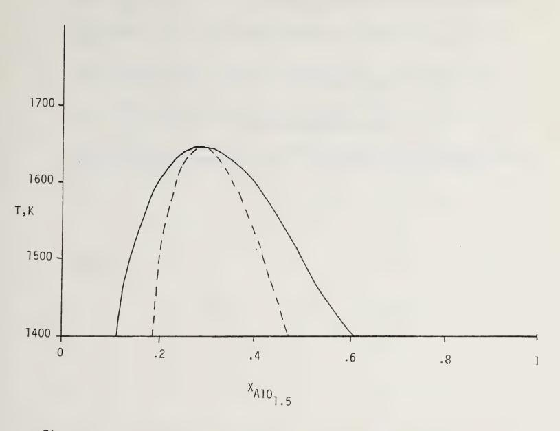
Figure 3.--Calculated curves for liquid-liquid immiscibility in metastable A10<sub>1.5</sub>-Si0<sub>2</sub> glasses. The dotted line shows the positions of maxima and minima in the activities.
