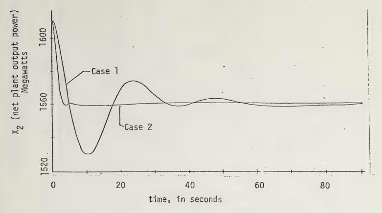
Figure 6. Net plant output power with heat capacitor
