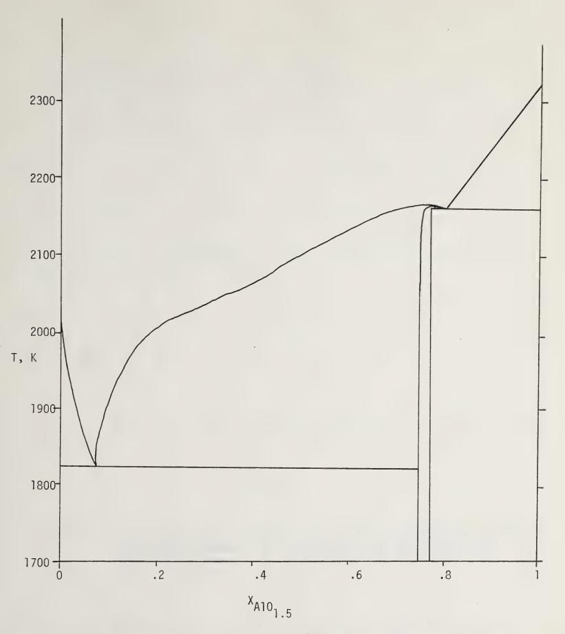
Figure 2.--Metastable AlO<sub>1.5</sub>-SiO<sub>2</sub> phase diagram, calculated omitting the gamma alumina phase. Note that mullite melts congruently just above the mullite-corundum eutectic.
