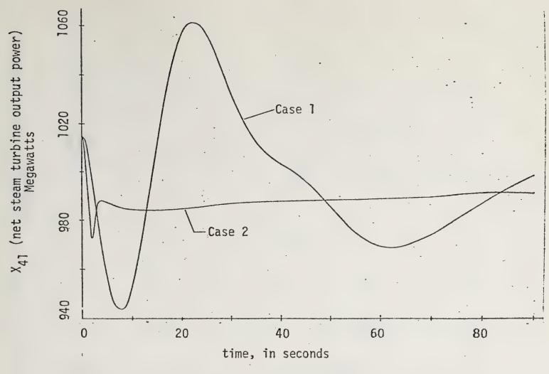
Figure 8. Net steam turbine output power with heat capacitor
