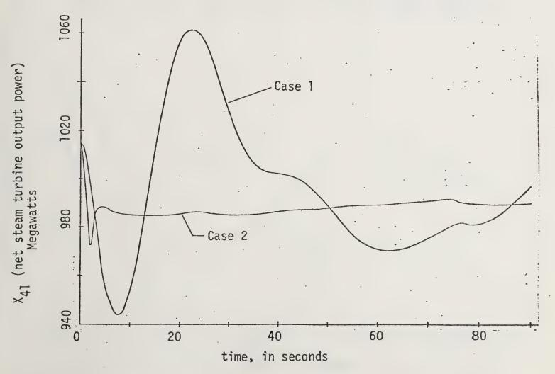
Figure 9. Net steam turbine output power without heat capacitor
