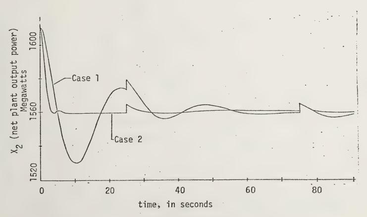
Figure 7. Net plant output power without heat capacitor
