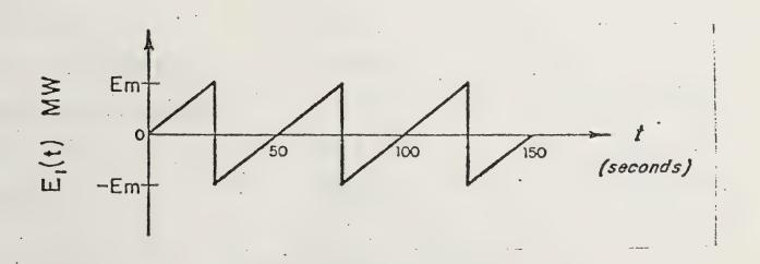
Figure 5. Thermal power variations at heat exchanger exit during reheat
