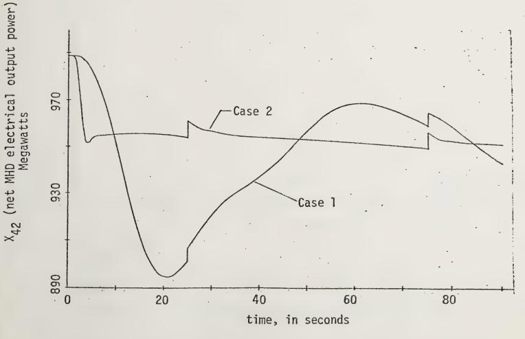
Figure 11. Net MHD electrical output without heat capacitor
