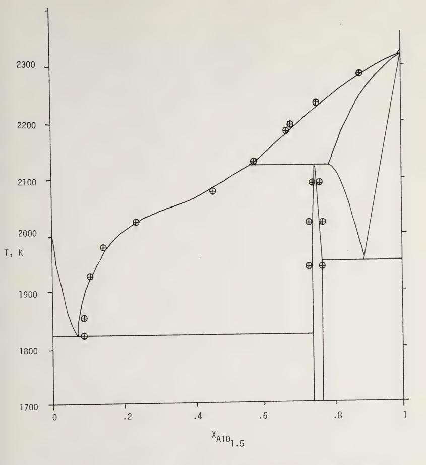
Figure 1.--Calculated AlO<sub>1.5</sub>-SiO<sub>2</sub> phase diagram. This shows a substantial region of stability for solutions of SiO<sub>2</sub> in gamma alumina, and an incongruent melting point for mullite. The circles represent experimental points of Davis and Pask and Aksay and Pask.
