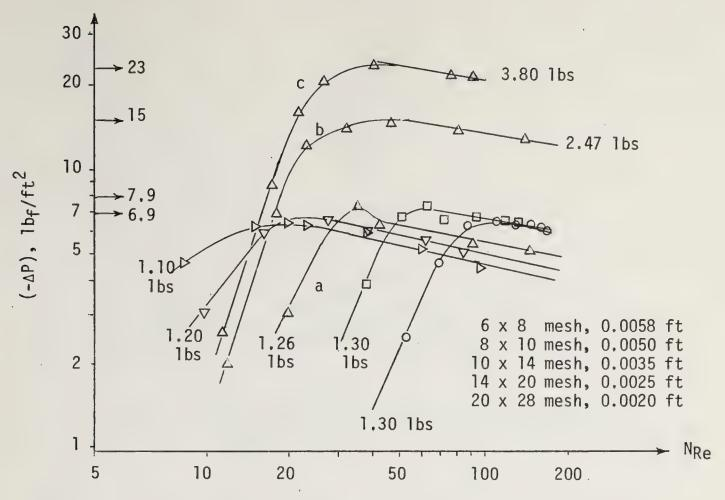
Figure 2. Batch fluidization curves for Rosebud coal in a 6-inch column at room temperature with a 5 percent open area orifice plate.
