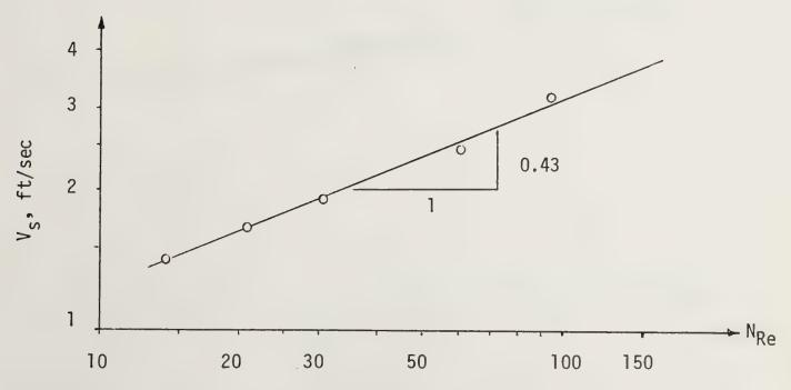
Figure 3. Superficial velocities at incipient fluidization. See Table 2.
