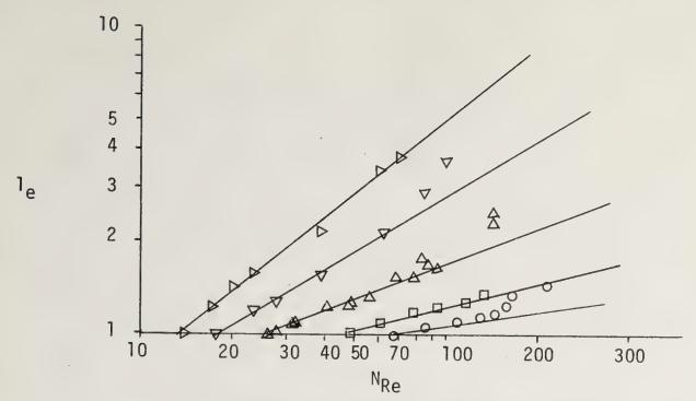
Figure 4. Correlation of bed expansion ratio, l<sub>e</sub>, with particle Reynolds Number. See Figure 2 for symbols.
