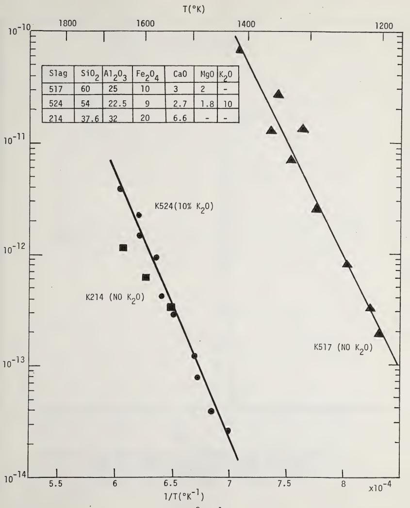
Figure 1.--Richardson plots  $(j/T^2 \text{ vs } \frac{1}{T})$  for three samples of synthetic slag
