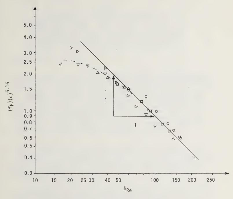
Figure 6. Correlation of fluidization friction factor and particle Reynolds Number for Rosebud seam coal.
