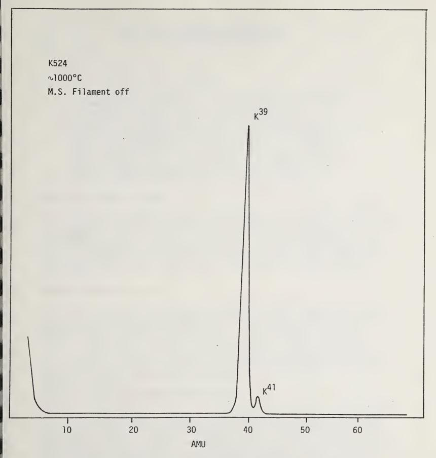
Figure 2.--Mass spectrometer trace measuring the ions emitted from slag K524 (The ionizer filament was turned off so that only ions emitted from the slag and entering the mass spectrometer are detected.)
