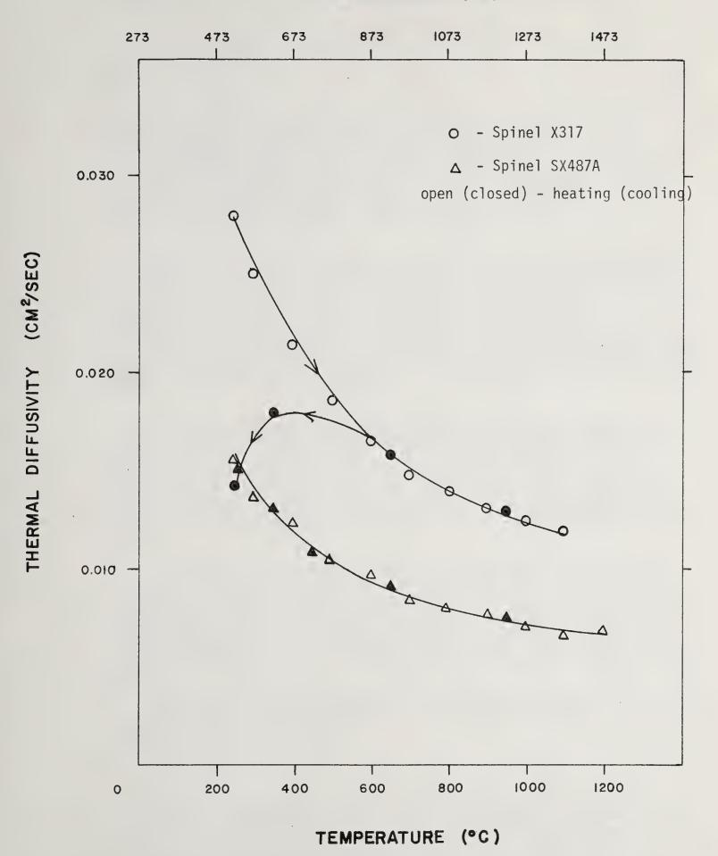
Figure 1. Thermal diffusivities of two as-fabricated magnesia aluminate refractories
