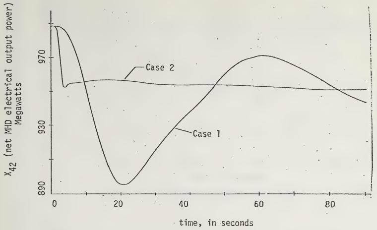
Figure 10. Net MHD electrical output with heat capacitor
