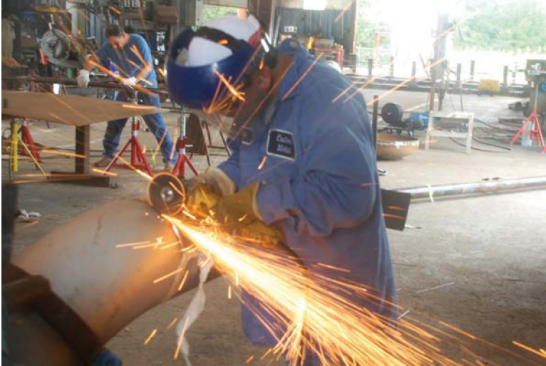
Figure 7.1 Alloy chemical process piping being prepared for welding away from the process hazards in a welding shop. Courtesy of Custom Metal, Lake Charles, LA.
