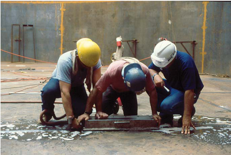
Figure 12.15 Inspectors using a vacuum box and soapy water to check for porous welds or other leaks on the welds on the floor of a low-pressure storage tank.
