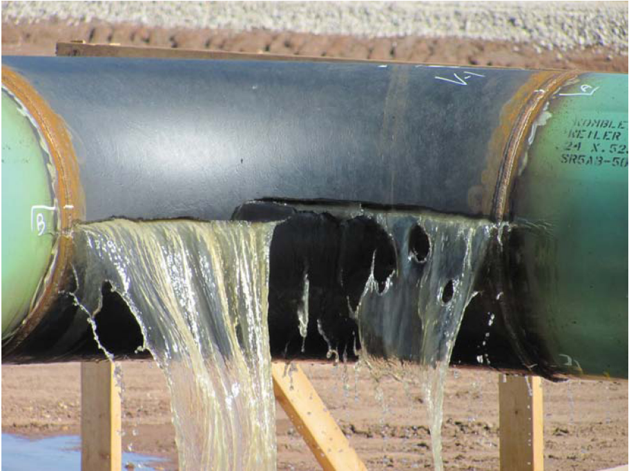
Figure 12.18 A close-up of the inferior, poorly manufactured 24-in. piping elbow which failed during a routine hydrotest.
