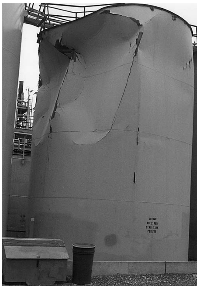
Figure 2.13 A 12-ft.-diameter storage tank ruined after vent system is improved.
