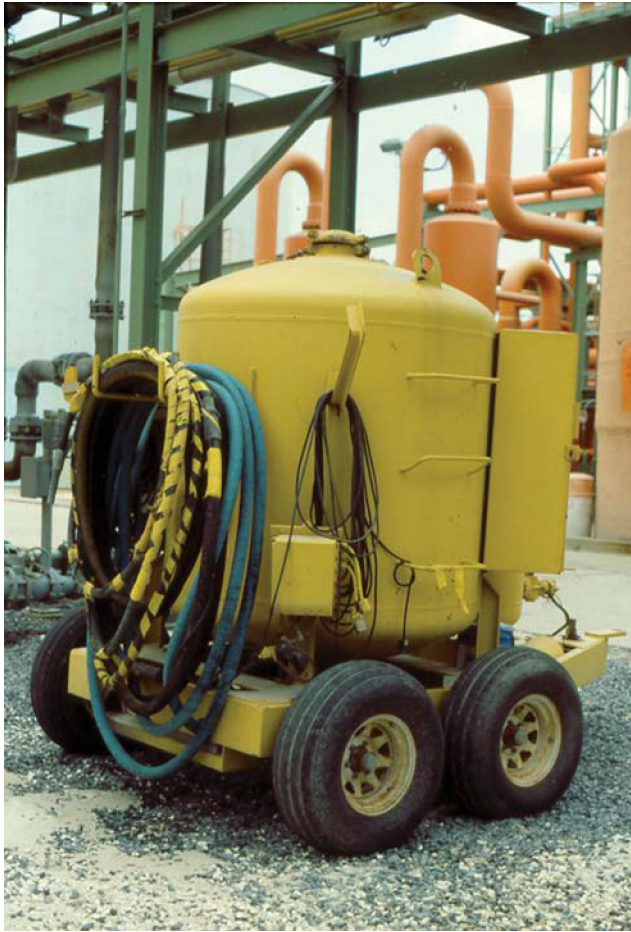
Figure 10.6 Repairs to a portable sandblast pot did not meet specifications and the lid pops off.
