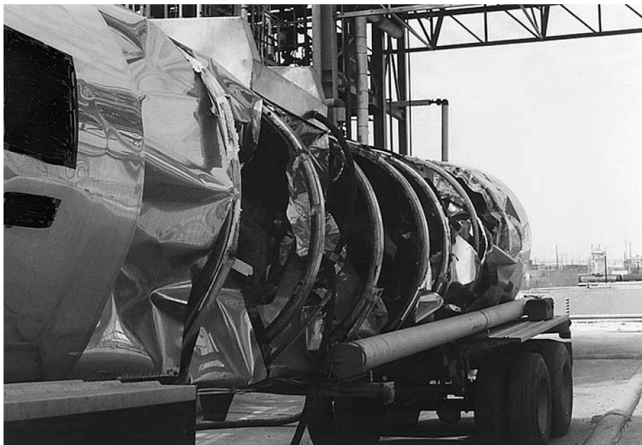
Figure 2.5 Closeup of tank failure and exposed ribs.
