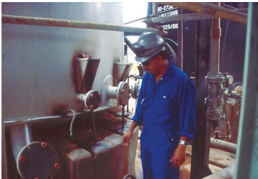
Figure 3.3 Tank bottom is bulged during a faulty hydro-test.
