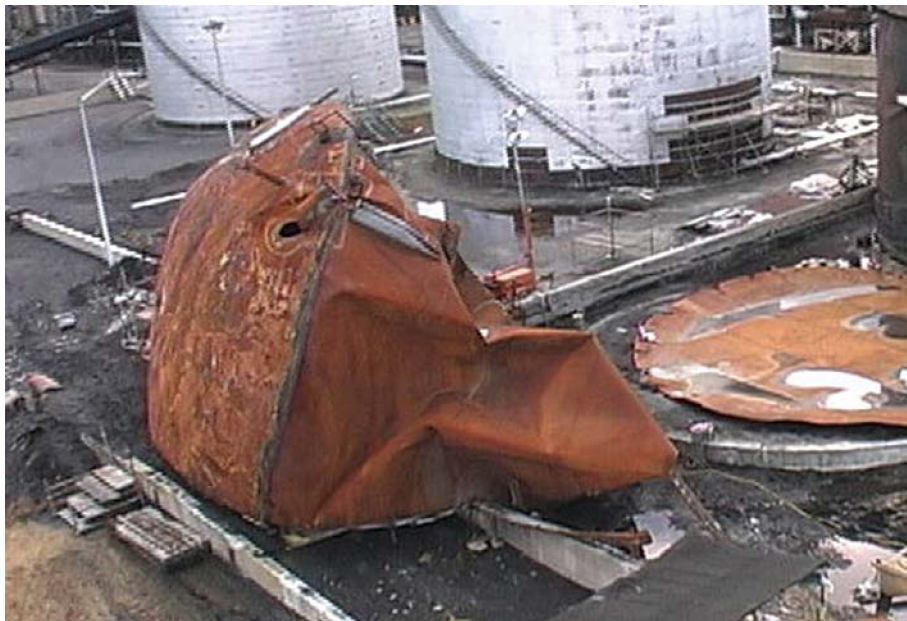
Figure 7.4 Sulfuric acid tank is destroyed during catwalk maintenance. Note the tank floor to the right and the fact that the typical weak roof design failed. Courtesy of Chemical Safety Board Report 2001-05-I-DE.
