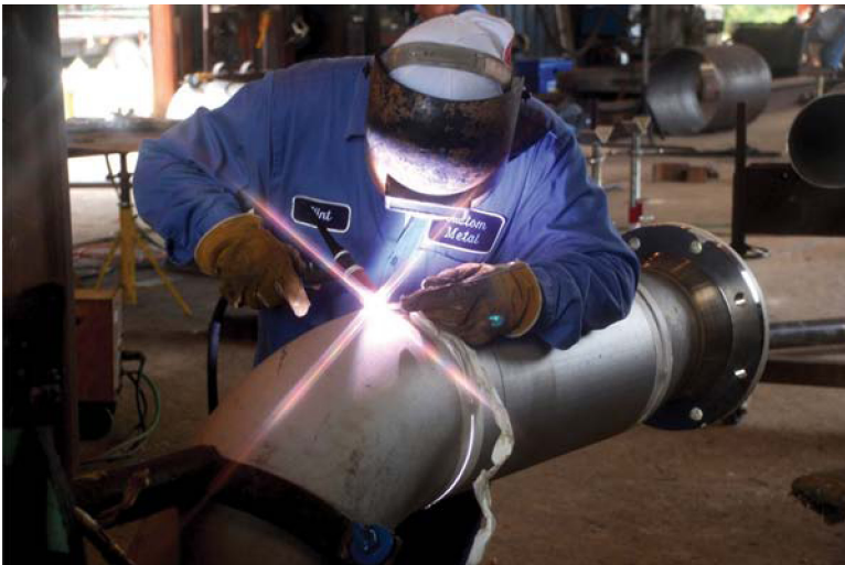
Figure 7.2 Alloy chemical process piping being welded to code specifications in a welding shop. Courtesy of Custom Metal, Lake Charles, LA.
