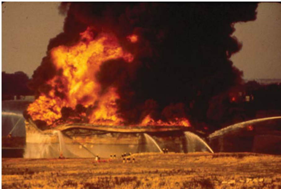
Figure 10.4 A huge tank fire confined by tank walls. This gigantic vessel is about 100 meters in diameter and after the fire started the burning liquid remains contained. Look hard and you will see at least eleven firefighters near the vessel attempting to control the blaze. Courtesy of the Institution of Chemical Engineers – from Hazard Workshop No. 3, “Fires and Explosions [8].”
