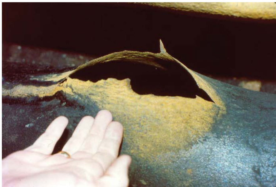
Figure 8.4 Close-up on the heat swollen tube and rupture of the fired heater tube.
