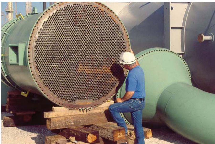
Figure 12.8 Qualified equipment inspectors play a key role inspecting equipment during fabrication in shops and after they are delivered. Here an inspector examines a retubed heat exchanger when it arrived at the plant site.
