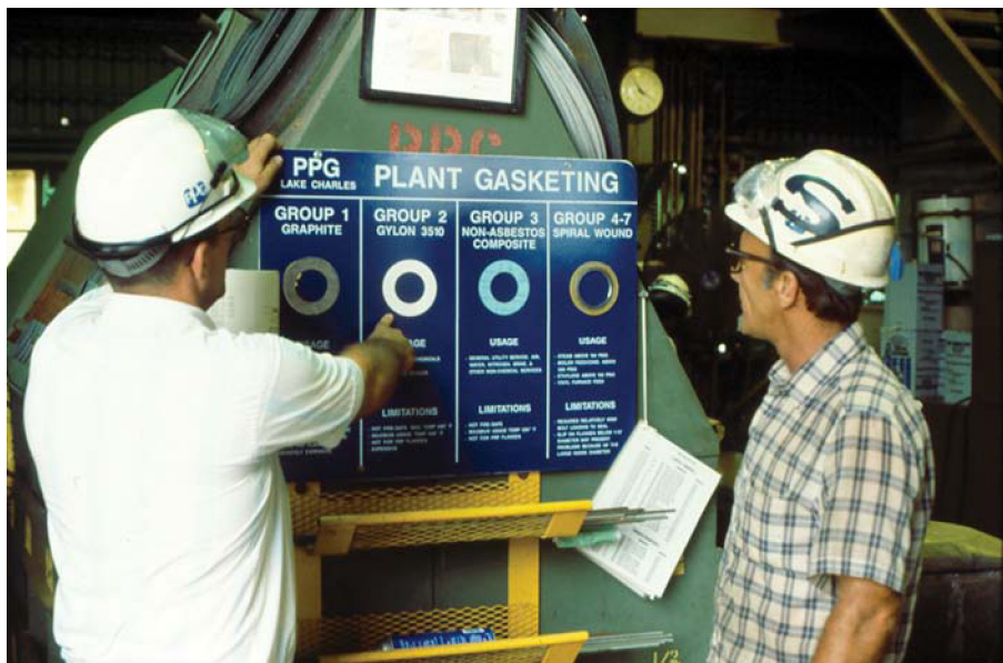
Figure 8.10 Choosing the proper piping gaskets is essential for process safety. A helpful easy-to-understand gasket board facilitates the selection.
