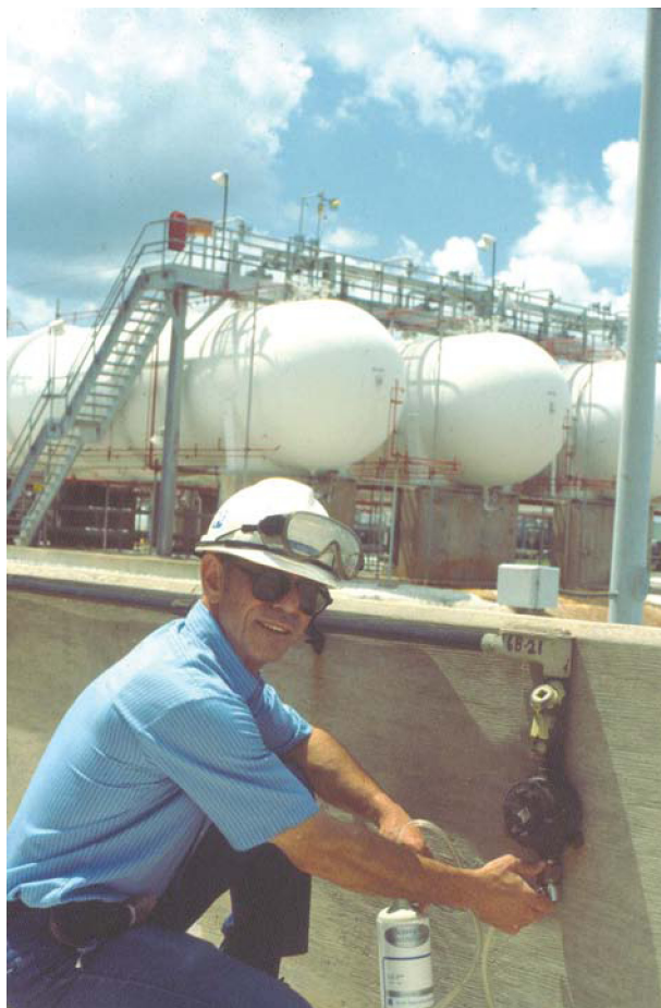
Figure 12.27 An instrument mechanic prooftesting a flammable vapor detector in a tank farm.
