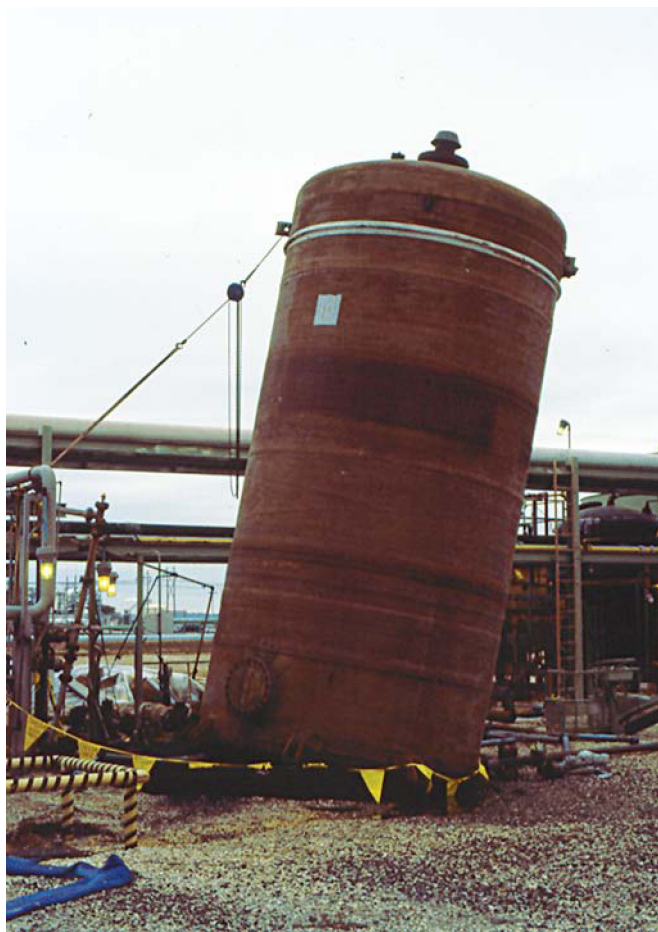
Figure 7.16 A large fiberglass acid tank fails due to blinded vent line and blinded overflow line.
