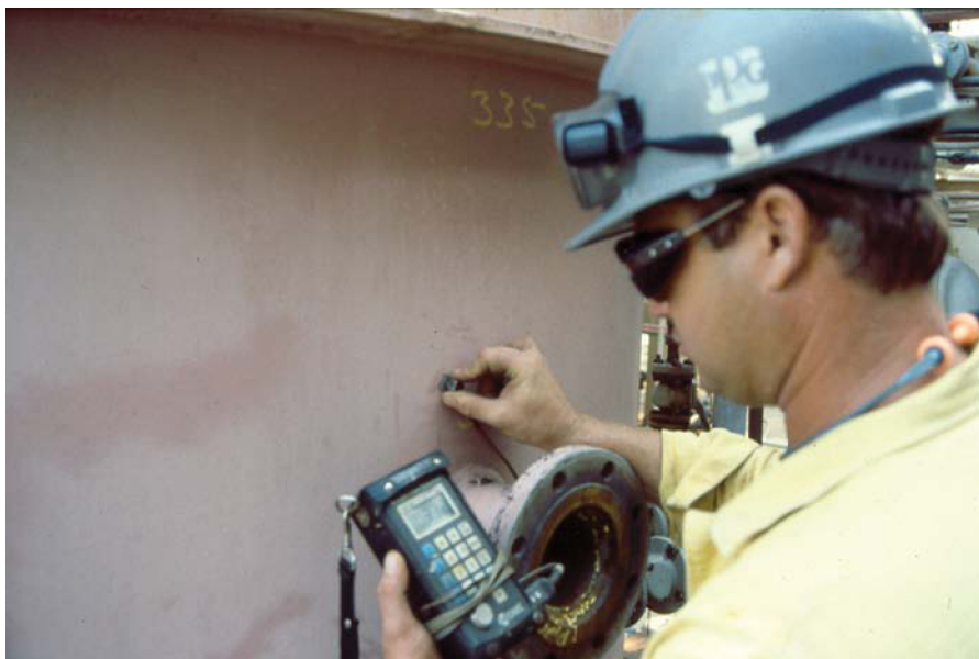
Figure 12.13 A certified pressure vessel inspector verifies the wall thickness on a vessel near a nozzle that had experienced significant metal loss.
