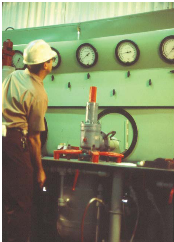
Figure 12.23 A mechanic trained as SRV Test Specialist, tests the relieving pressure of the safety relief valve just as it was received from the operating unit.
