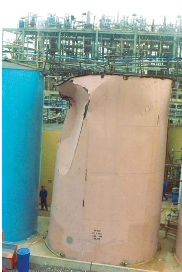
Figure 2.16 Tank collapsed during pump out and was destroyed beyond repair.
