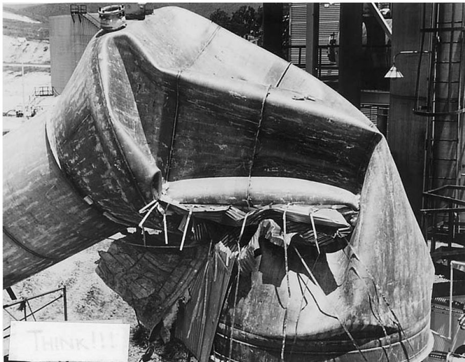
Figure 3.7 A close-up of a collapsed stripper column base. Courtesy of Guido DeJesus.
