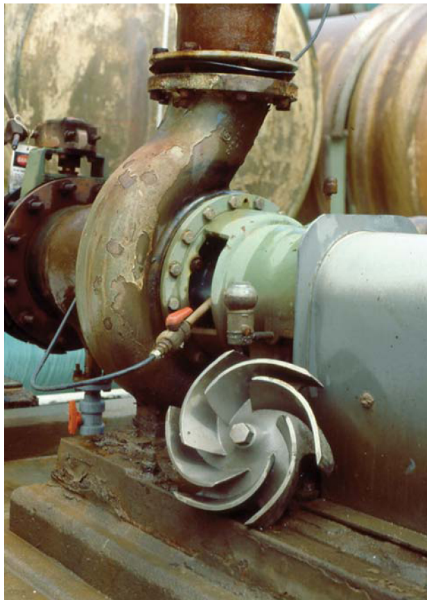
Figure 10.12 Brine pump received an out of spec impeller – trace chrome in the brine stream could have created an explosion in the chlorine manufacturing cells.
