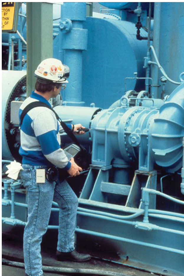
Figure 12.3 A technician gathering vibration readings from a refrigeration compressor to help ensure reliability.
