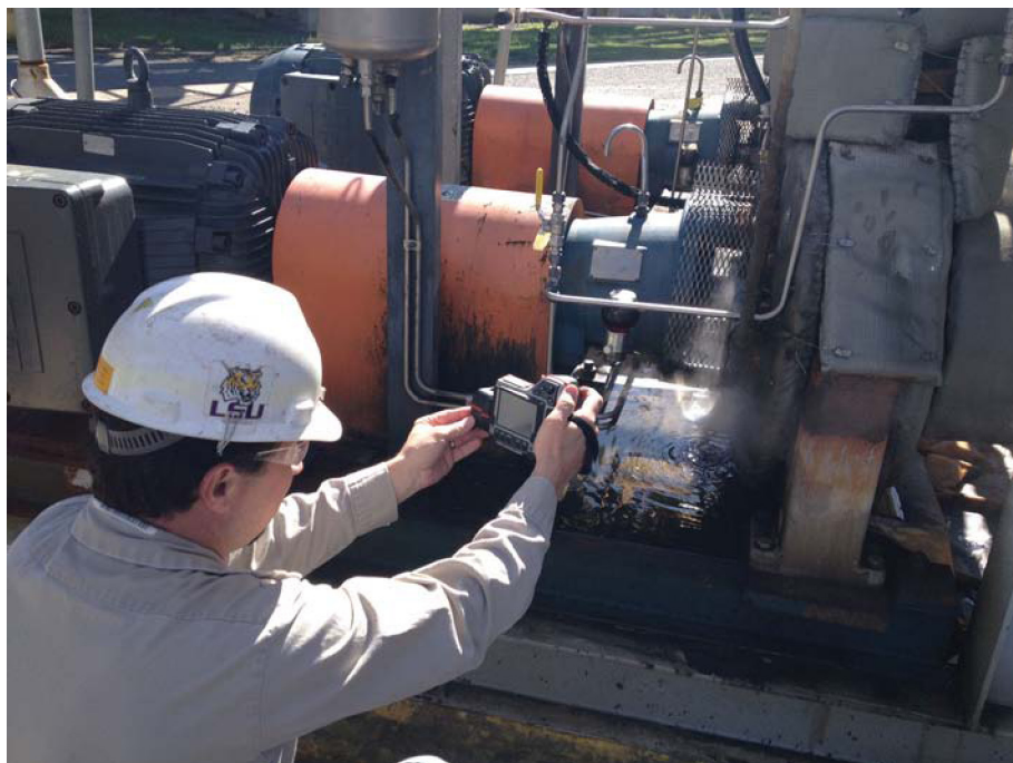
Figure 12.5 Thermography survey – an engineer taking infrared readings on a hot oil pump including a look at the bearings and the insulation.
