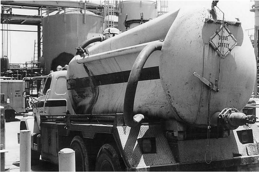
Figure 12.14 A collapsed service company vacuum truck tank signals an inadequate mechanical integrity program.
