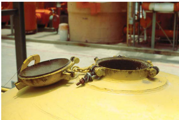
Figure 10.7 A close-up look at the quick closure bolts that failed on the sand pot.
