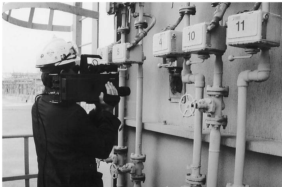
Figure 12.6 An Inspector uses an infrared camera to periodically monitor furnace tube temperatures via the port holes. The objective is to look for potential hot spots which will indicate coking within the tubes and damage to the tubes.
