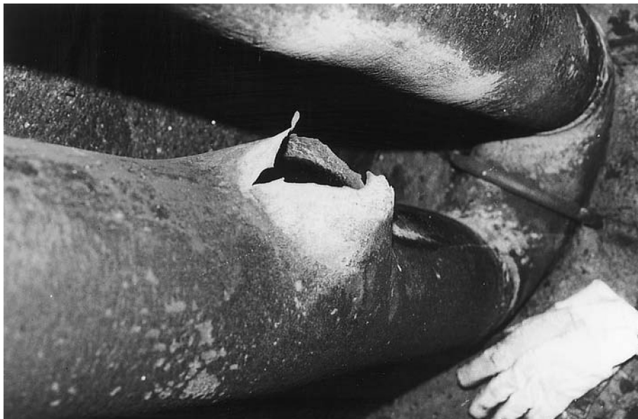
Figure 8.3 Classical tube rupture of a fired heater from flame impingement on a blocked-in heater tube.
