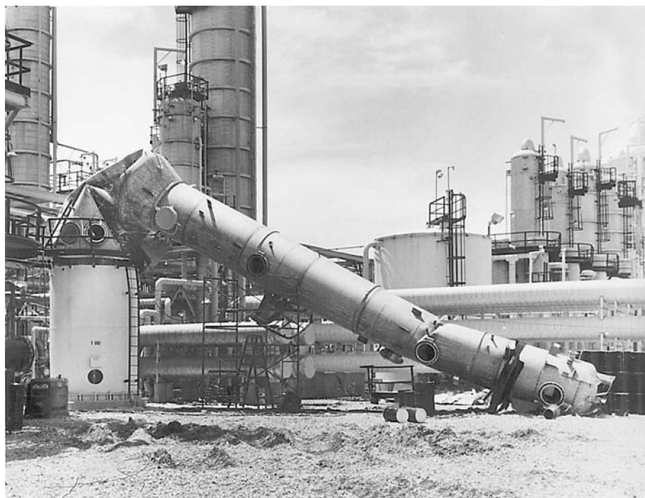
Figure 3.5 A stripper column collapses when water is pumped out. Courtesy of Guido DeJesus.
