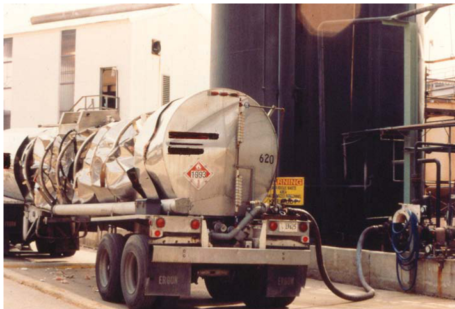
Figure 2.2 Collapsed tank truck with unloading hose connected.
