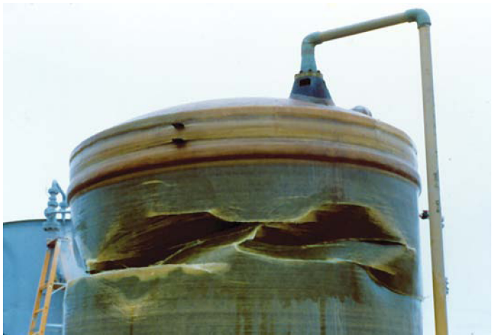
Figure 2.9 Closeup of collapsed acid tank.
