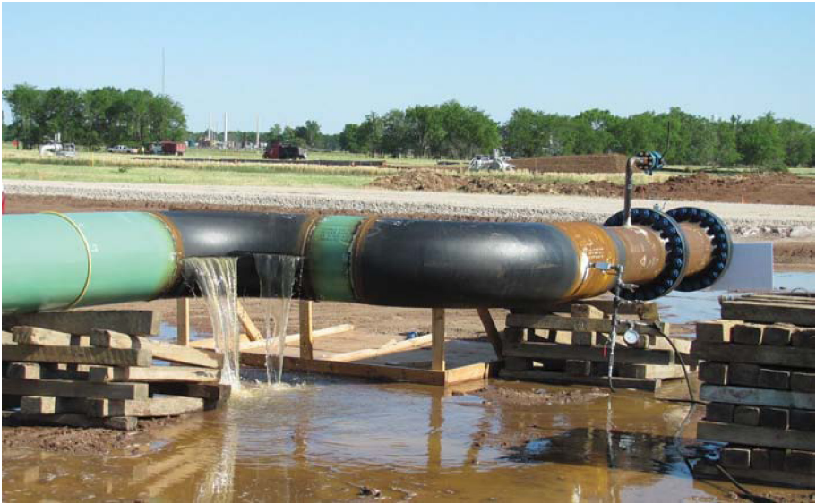
Figure 12.17 Fabricated piping should be tested prior to conveying hazardous materials. Usually piping is hydrotested. This is a rare failure of a 24-in. piping elbow.
