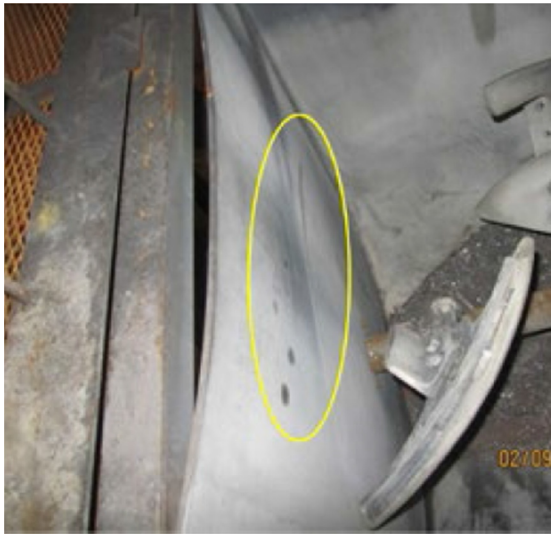
Fig. 21 Blender wall deformation and indications of blade scraping (thus effectively completing the explosion pentagon) at AL Solutions facility (CSB, 2014c).
