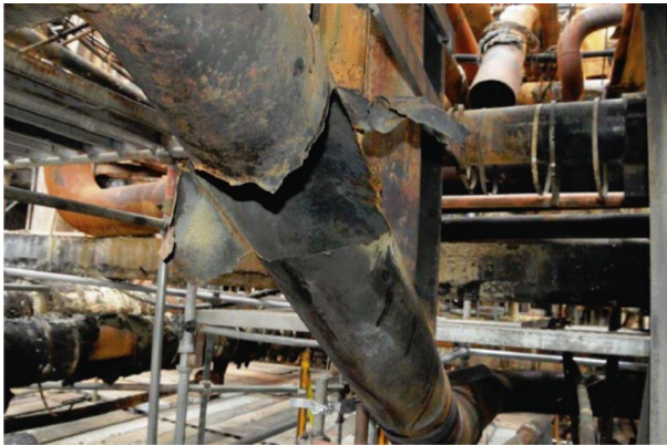
Fig. 18 Pipeline degradation due to sulfidation corrosion at Chevron Richmond refinery (CSB, 2013).
