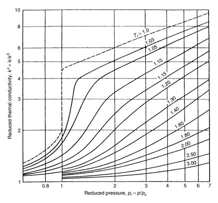
**Figure 1-8.** Modified reduced thermal conductivity as a function of reduced temperature and pressure. (Reproduced with permission from reference 5. Copyright 1953, American Institute of Chemical Engineers.)
