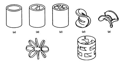
Figure 13-5. Random tower packings. (Adapted from reference 4.)
