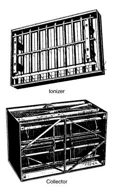
Figure 14-20. Electrostatic precipitator. (Adapted from reference 5.)
