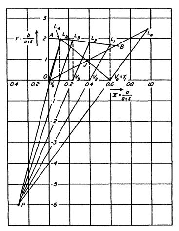
**Figure 13-23.** Equilibrium diagram and solution for Example 13-6. (Adapted from reference 6.)
