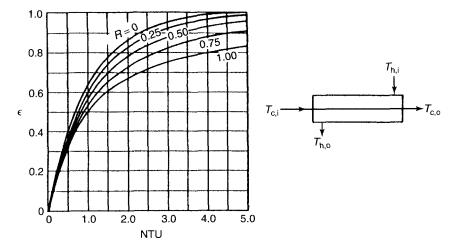
Figure 8-9. Counterflow heat exchanger effectiveness relation (4). (With permission of W. M. Kays.)
