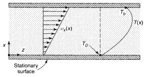
**Figure 5-6.** Physical analog to rotating cylinders with viscous dissipation. (Reproduced with permission from reference 6. Copyright 1960, John Wiley and Sons.)
