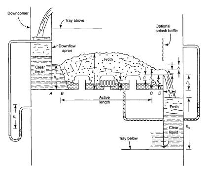
Figure 12-17. Bubble cap tray fluid dynamics (19).
