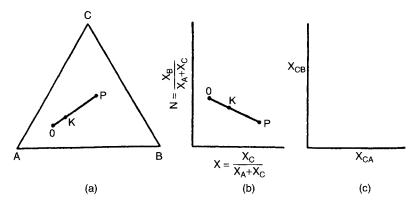
Figure 13-10. Comparison of ternary, Janecke, and distribution diagrams (5).
