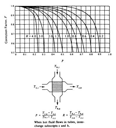
**Figure 8-7.** *F* factor for single pass cross-flow exchanger (one fluid mixed). (Reproduced with permission from reference 3. Copyright 1940, American Society of Mechanical Engineers.)
