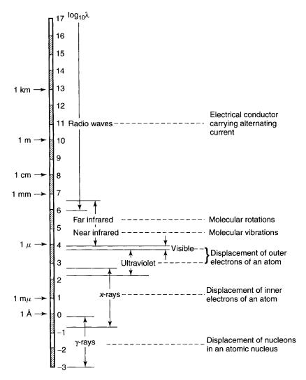
**Figure 9-1.** Spectrum of electromagnetic energy. (Adapted with permission from reference 9. Copyright 1960, John Wiley and Sons.)
