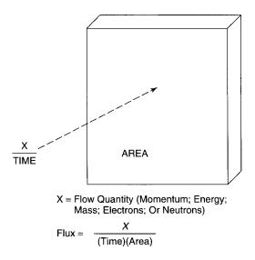
Figure 1-1. Schematic of a flux.
