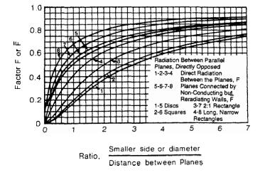
Figure 9-4. Radiation shape factors between parallel planes (1).
