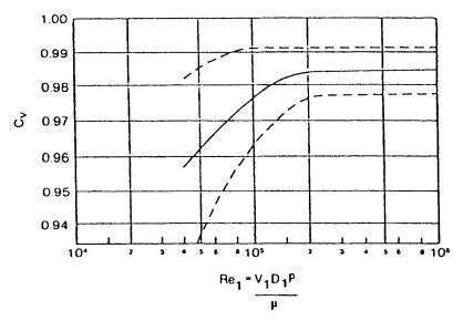
**Figure 2-23.**  $C_v$  data for Venturi meters. (Adapted with permission from reference 7. Copyright 1959, American Society of Mechanical Engineers.)
