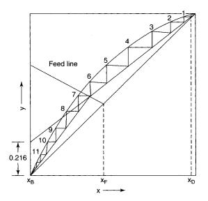
**Figure 12-25.** Solution for feed that is two-thirds vapor. (Reproduced with permission from reference 18. Copyright 1997, American Chemical Society.)
