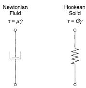
**Figure 2-12.** Ideal elastic solid spring model. Newtonian liquid dashpot model. (Adapted from reference 4 with permission of J. M. McKelvey.)
