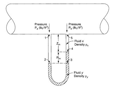
Figure 2-4. Manometer in pipeline.
