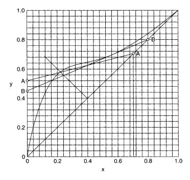
Figure 12-29. Equilibrium diagram for Example 12-6. (Adapted from reference 12.)
