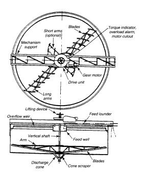
Figure 14-17A. Gravity thickener. (Courtesy of Eimco Corporation.)
