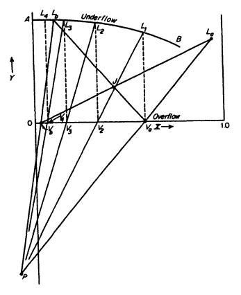
Figure 13-18. Solution for leaching stages. (Adapted from reference 6.)
