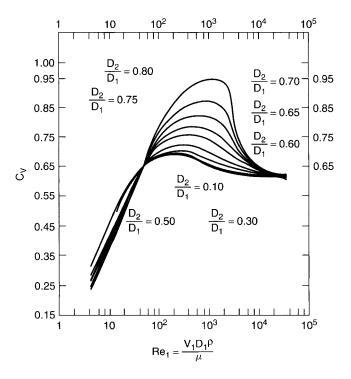
**Figure 2-24.**  $C_v$  Data for orifice meters. (Adapted from reference 8.)
