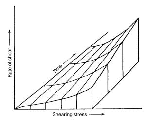
**Figure 2-15.** Rheopectic fluid behavior. (Adapted with permission from reference 5. Copyright 1963, John Wiley and Sons.)
