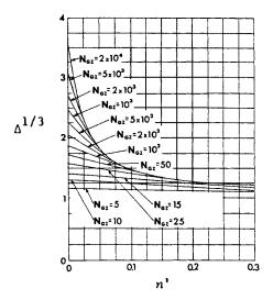
**Figure 7-2.** Factor  $\Delta^{1/3}$  for laminar flow and low *n* values. (Reproduced with permission from references 3–5. Copyright 1957, American Institute of Chemical Engineers. Copyrights 1960 and 1964, *Chemical Engineering Science*.)
