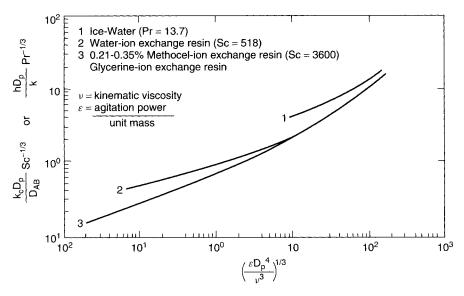
**Figure 11-4.** Heat and mass transfer analogy for solid particles suspended in an agitated fluid. (Adapted with permission from references 9 and 11. Copyright 1969 and 1962, American Institute of Chemical Engineers.)
