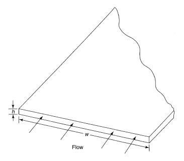
Figure 3-8. Flow between parallel plates.
