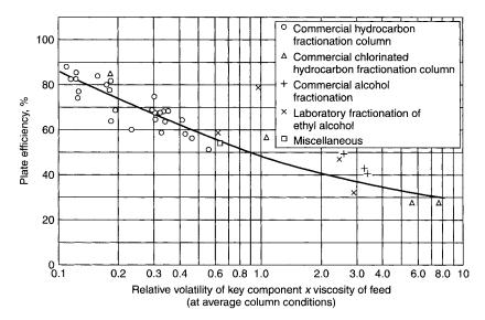
**Figure 12-22.** O'Connell correlation for overall efficiency. (Reproduced with permission from reference 16. Copyright 1946, American Institute of Chemical Engineer.)
