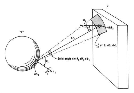
**Figure 9-2.** Radiation system model. (Adapted with permission from reference 9. Copyright 1960, John Wiley and Sons.)
