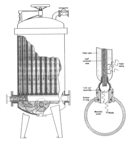
**Figure 14-5.** Vertical leaf filter and filter leaf. (Courtesy of Industrial Filter and Pump Mfg. Co.)
