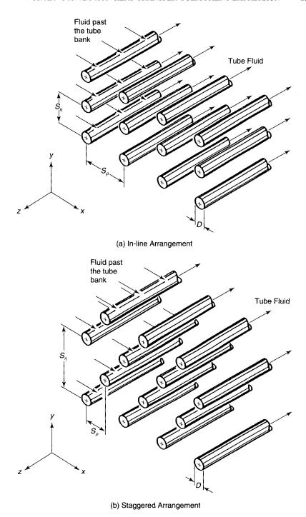
Figure 6-4. In-line and staggered tube arrangements. (Adapted from reference 21.)
