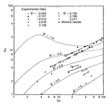
**Figure 7-3.** Nusselt–Graetz relationship for molten or thermally softened flowing polymers with viscous dissipation and thermal expansion effects. (Reproduced with permission from references 6 and 7. Copyrights 1972 and 1975, Society of Plastics Engineers.)
