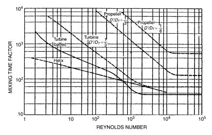
**Figure 4-8.** Mixing time factor (*N* times mixing time) as a function of Reynolds number. (Reproduced with permission from references 9 and 10. Copyright 1966 and 1972, American Institute of Chemical Engineers.)
