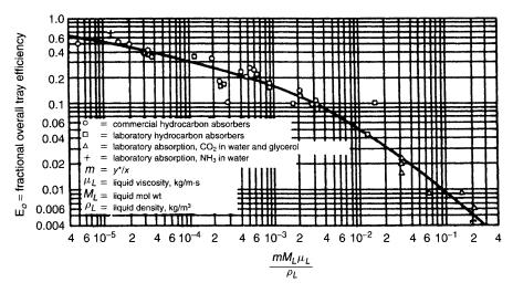
**Figure 13-19.** Overall efficiencies for bubble cap towers. (Reproduced with permission from reference 10. Copyright 1946, American Institute of Chemical Engineers.)
