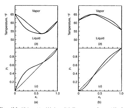
**Figure 12-5.** Minimum (a) and Maximum (b) boiling azeotropes. System a (chloroform 1, and methanol 2 system b (acetone 1, and chloroform, 2) (19).
