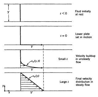
**Figure 1-3.** Velocity profile development for steady laminar flow. (Adapted with permission from reference 1. Copyright 1960, John Wiley and Sons.)
