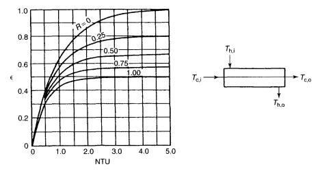
Figure 8-8. Parallel flow heat exchanger effectiveness relation (4). (With permission of W. M. Kays.)
