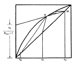
**Figure 12-12.** Infinite stages and minimum reflux with intersection of equilibrium curve feed line and rectifying mass balance. (Reproduced with permission from reference 18. Copyright 1997, American Chemical Society.)
