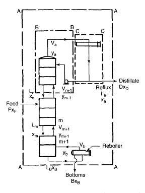
**Figure 12-7.** Schematic of a continuous distillation column. (Reproduced with permission from reference 18. Copyright 1997, American Chemical Society.)
