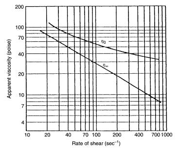
**Figure 2-14.** Thixotropic fluid behavior. No is initial viscosity:  $\eta_0$  is initial viscosity;  $\eta_\infty$  is viscosity after infinite time. (Adapted with permission from reference 5. Copyright 1963, John Wiley and Sons.)
