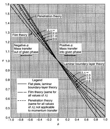
**Figure 11-6.** Correction of mass transfer coefficients, heat transfer coefficients, and friction factors due to high mass transfer rates. (Reproduced with permission from reference 21. Copyright 1960, John Wiley and Sons.)
