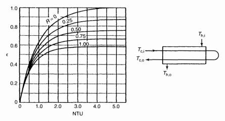
Figure 8-12. Relation for effectiveness (1-2 parallel counterflow exchangers) (4). (With permission of W. M. Kays.)
