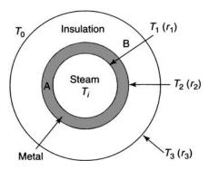
Figure 8-1. Combined conduction and convection (1).
