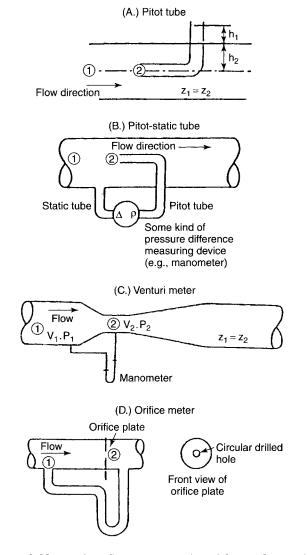
Figure 2-22. Various flow meters. (Adapted from reference 3.)
