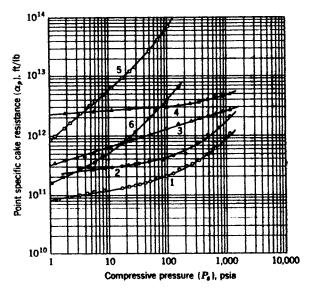
**Figure 14-2.** Point specific cake resistance versus compressive pressure. Codes: 1, 2 Superlite CaCO, pH values of 9.8 and 10.3; 3, 4 TiO, pH values of 7.8 and 3.5; 5,6 ZnS, pH values of 9.1. Curves 1, 3 for flocculated systems. (Reproduced with permission from reference 1. Copyright 1953, American Institute of Chemical Engineers.)
