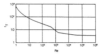
**Figure 4-7.** Mixing times as a function of Reynolds numbers for miscible fluids in turbine agitated vessels. (Reproduced with permission from reference 7. Copyright 1960, American Institute of Engineers.)
