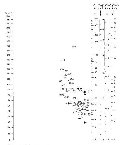
**Figure B-5.** Liquid Prandtl numbers. (Reproduced with permission from reference 8. Copyright 1997, American Chemical Society.)
