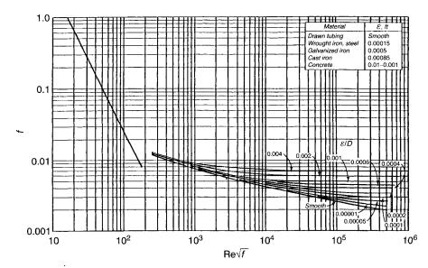
**Figure 3-12.** Modified friction factor plot. (Reproduced with permission from reference 8. Copyright 1997, American Chemical Society.)
