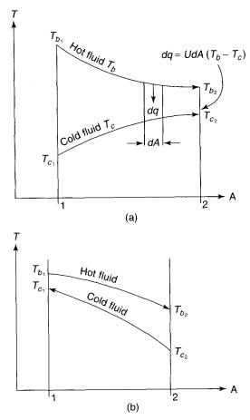
Figure 8-2. Temperature behavior in parallel (a) and counterflow (b) systems. (Reproduced with permission from reference 2. Copyright 1997, American Chemical Society.)
