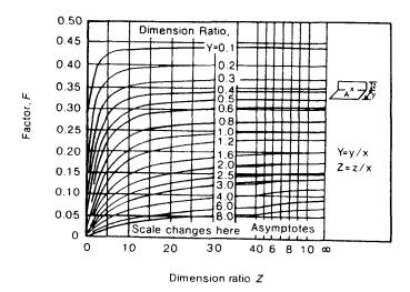
Figure 9-3. Radiation shape factors between adjacent surfaces (1).
