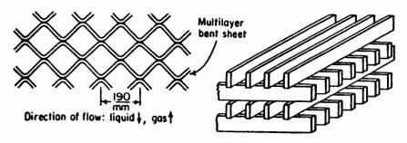
Figure 13-6. Stacked packings. (Adapted from reference 4.)
