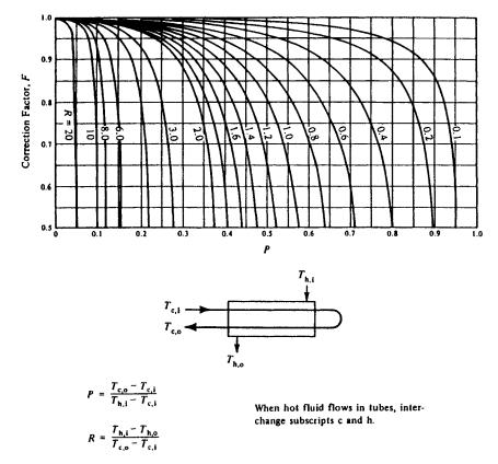
**Figure 8-4.** F factor for one shell pass and any multiple of tube passes. (Reproduced with permission from reference 3. Copyright 1940, American Society of Mechanical Engineers.)
