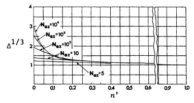
**Figure 7-1.** Factor  $\Delta^{1/3}$  for laminar flow. (Reproduced with permission from references 3–5. Copyright 1957, American Institute of Chemical Engineers. Copyrights 1960 and 1964, *Chemical Engineering Science*.)
