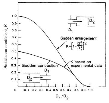
**Figure 3-6.** Sudden expansion and contraction resistances. (Adapted from reference 5. Permission of Crane Co. Copyright, all rights resolved.)
