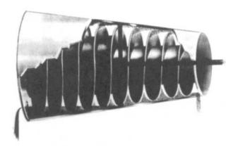
Figure 14-13. Solid bowl centrifuge. (Courtesy of Sharples Corp.)
