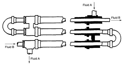
**Figure 8-3.** Double-pipe heat exchanger. (Reproduced with permission from reference 2. Copyright 1997, American Chemical Society.)
