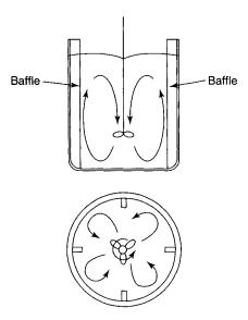
Figure 4-4. Baffled agitator system (8).
