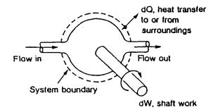
Figure 2-20. First law flow system. (Adapted from reference 3.)
