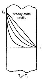
**Figure 5-1.** Unsteady (curves) and steady-state (straight line) temperature profiles in a slab. (Reproduced with permission from reference 5. Copyright 1997, American Chemical Society.)
