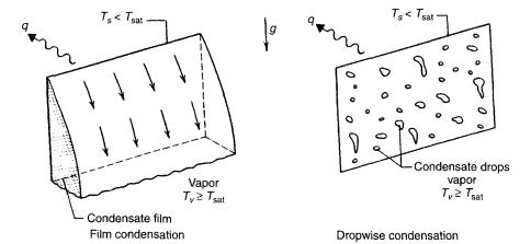
**Figure 7-4.** Laminar condensate film on vertical surface (24). Film and dropwise condensation on a vertical surface (Adapted with permission from reference 25. Copyright 1981, John Wiley and Sons Inc.)
