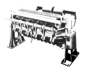
Figure 14-7. Sweetland pressure filter. (Courtesy of GL & V/Dorr-Oliver.)
