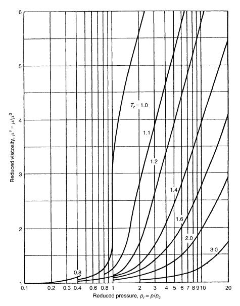
**Figure 1-6.** Modified reduced viscosity as a function of reduced temperature and pressure (3). (Trans. Am. Inst. Mining, Metallurgical and Petroleum Engrs *201* 1954 pp 264 ff; N. L. Carr, R. Kobayashi, D.B. Burrows.)
