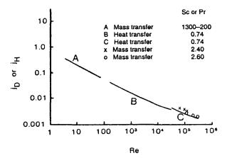
**Figure 11-5.** Mass and heat transfer for normal flow to a cylinder. (Curve A, with permission from reference 14. Curves B and C, data with permission from references 12, 13, and 15. Copyright 1940, 1969, 1970, American Society of Mechanical Engineers.)
