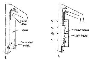
**Figure 14-15.** Tubular bowl centrifuge internal configurations for solid-liquid and liquid-liquid separations. (Adapted with permission from reference 2. Copyright 1960, John Wiley and Sons, Inc.)
