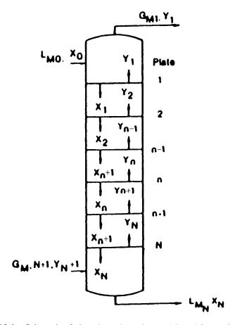
Figure 13-1. Schematic of plate absorption column, (Adapted from reference 3.)
