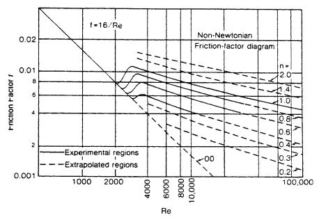
**Figure 4-3.** Friction factor versus modified Reynolds number for non-Newtonians. (Reproduced with permission from reference 5. Copyright 1959, American Institute of Chemical Engineers.)
