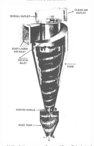
Figure 14-18. Cyclone separator. (Courtesy of Ducon Technologies, Inc.)
