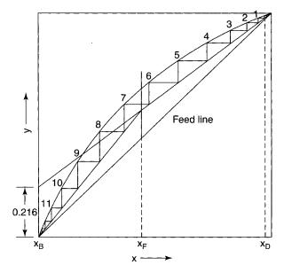
**Figure 12-23.** Solution for saturated liquid feed. (Reproduced with permission from reference 18. Copyright 1997, American Chemical Society.)
