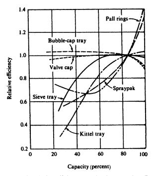
**Figure 13-20.** Contacting device efficiency as related to capacity. (Reproduced with permission from references 11 and 12. Copyright 1960, Institute of Chemical Engineers. Copyright 1963, Institute of Chemical Engineers.)
