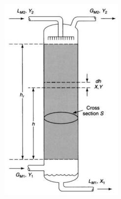
Figure 13-7. Schematic for packed column design. (Adapted from reference 3.)
