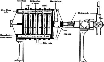
Figure 14-1. Plate and frame filter press. (Courtesy of T. Schriver and Co.)
