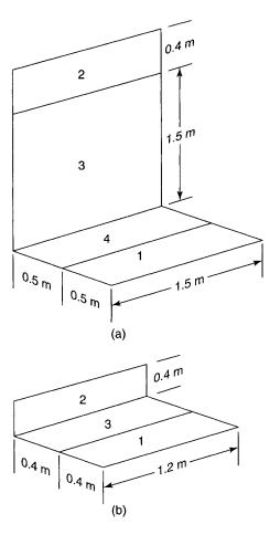
Figure 9-10. Radiation shape factor systems.
