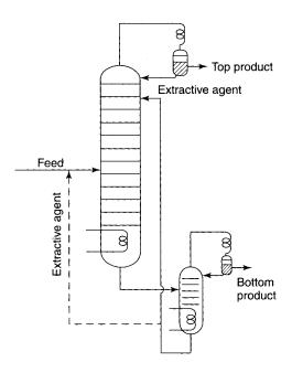
**Figure 12-16.** Extractive distillation system (11).
