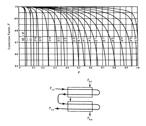
**Figure 8-5.** F factor for two shell passes and any multiple of tube passes. (Reproduced with permission from reference 3. Copyright 1940, American Society of Mechanical
