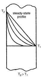
**Figure 1-2.** Temperature profile development (unsteady to steady state). (Reproduced with permission from reference 18. Copyright 1997, American Chemical Society.)
