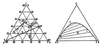
**Figure 13-9.** Ternary diagram. See that point M consists of 20 percent A, 40, percent B, and 40 percent C. Relative amounts of E and D in E are given by DE divided by EF. Line AG has constant ratios of E to E0 and varying amounts of E1. (Adapted from reference 5.)
