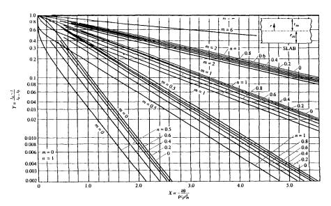
**Figure 5-3.** Temperature as a function of time and position in a slab. (Reproduced with permission from reference 3. Copyright 1923, American Chemical Society.)
