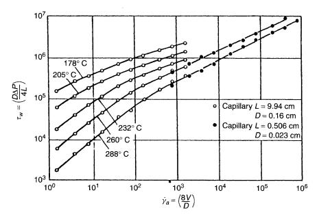
**Figure 4-2.** Logarithmic plot of  $(D\Delta P/4L)$  versus (8V/D). (Adapted from reference 4.)
