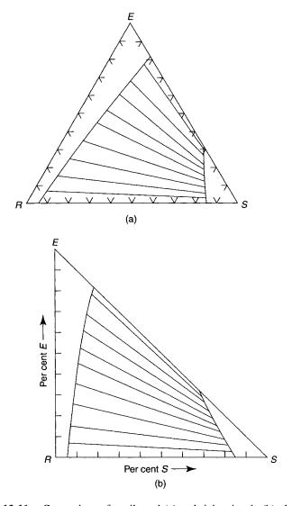
Figure 13-11. Comparison of equilateral (a) and right triangle (b) plots (55).
