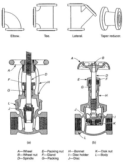
**Figure 3-4.** Pipe fittings. (a) Globe valve. (b) Gate valve. (Adapted with permission from reference 2. Copyright 1960, John Wiley and Sons.)
