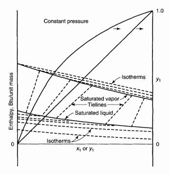
Figure 12-14. Construction of an enthalpy-composition plot (constant pressure) (19).
