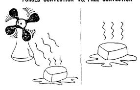
**Figure 6-2.** Examples of free and forced convection. (Reproduced with permission from reference 22. Copyright 1997, American Chemical Society.)
