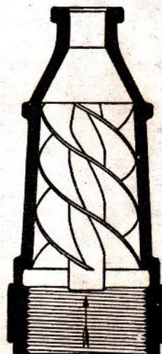
FIG. 526. Single-fluid pressure spray nozzle. (Schutte and Koerting Co.)
