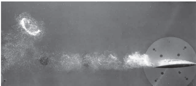
Figure 7.13 A vortex ring shed by the partial cavitation oscillations of a hydrofoil. The flow is from right to left. Reproduced with the permission of A.J. Acosta.
