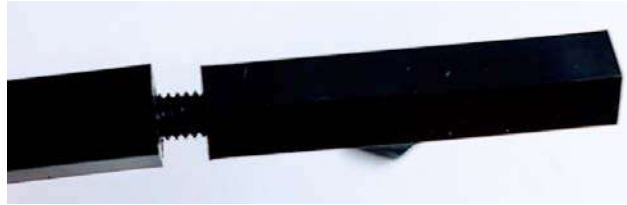
Figure 12.6 – Joining the standoff posts
