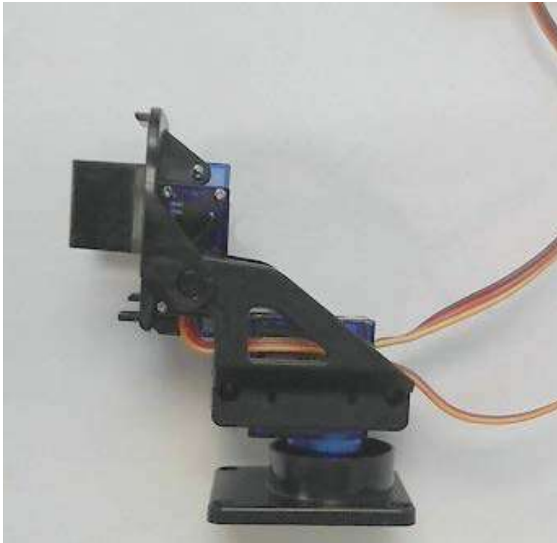
Figure 10.8 – A pan and tilt mechanism from a typical kit
