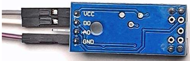
Figure 11.7 – The sensors with cable connections
