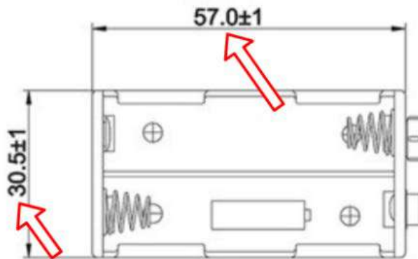
Figure 6.16 – A battery box product drawing with dimensions
