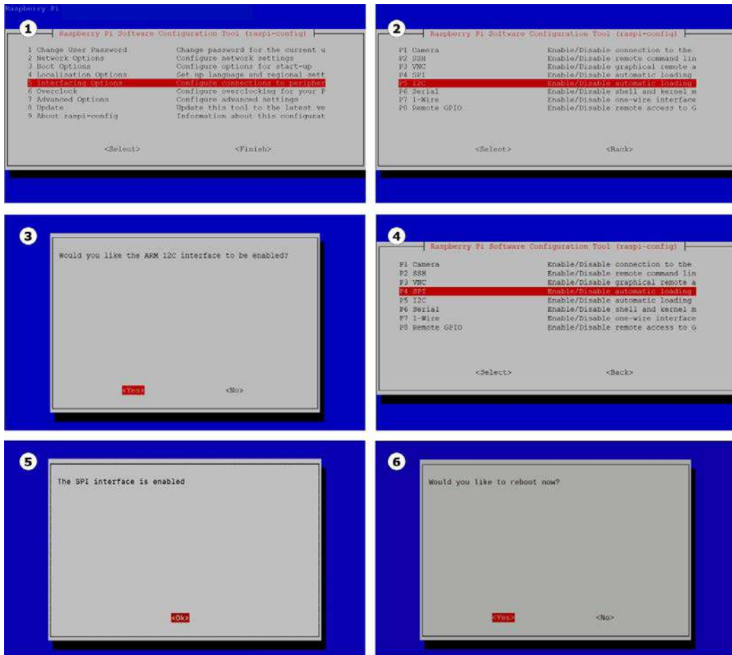
Figure 7.1 – Using raspi-config to enable SPI and I2C
