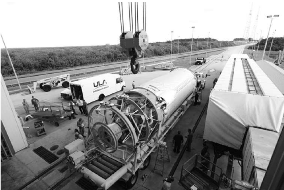
Figure 2.5 Photo of the Centaur upper stage using the RL 10 engine for propulsion being offloaded by NASA and ULA crew for NASA's Mars Science Laboratory (MSL) mission (Source: https://mars.nasa.gov/mars2020/multimedia/images/?ImageID=3638&s=6 ).
