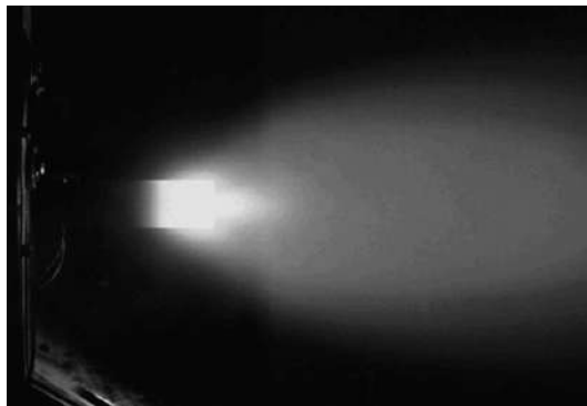
Figure 13.5 High-power ammonia arcjet firing shows hydrogen Balmer series recombination occurring in plume far downstream of nozzle exit (Image courtesy of Aerojet Rocketdyne).
