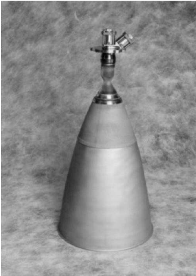
Figure 2.6 R-4D liquid apogee engine using storable bipropellant combination for orbit circularization and in-flight maneuvers (Source: Aerojet Rocketdyn).
