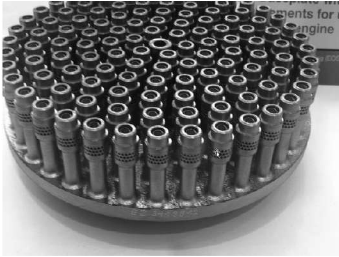
Figure 8.32 Ariane Vinci engine injector additively manufactured from a stainless steel alloy as a single part. The coaxial injector features 123 individual elements with hundreds of radial ports for gaseous hydrogen injection into individual elements.
